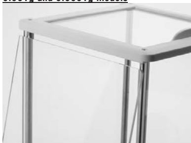
1) Install Side Doors - Insert fully into Top Frame then down over retainer.
